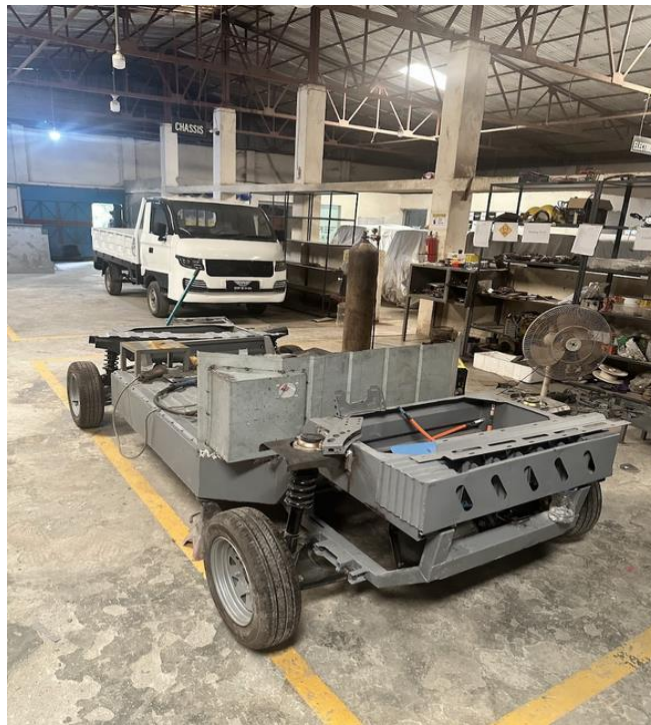
Chassis and drivetrain layout of the Cityboy platform, optimised for commercial ride-sharing use.
